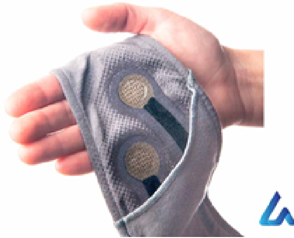
Figure 2: Textile electrode for ECG measurements (Source: [12]).
